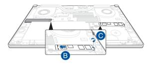
$\mbox{NOTE:}$  A second M.2 card module slot is only available on GTX 1660 Ti and RTX 2060 models.
